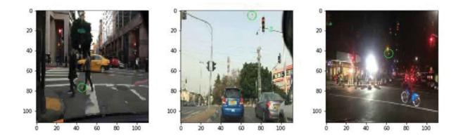
Source: Nexar Deep Learning Traffic Light Challenge. (a) Red light classified as green with 68% confidence after one pixel is changed. (b) Red light classified as green with 95% confidence after one pixel is changed. (c) Red light classified as green with 78% confidence after one pixel is changed.
