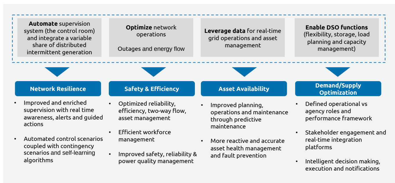
Figure 1: Functions of the control room
