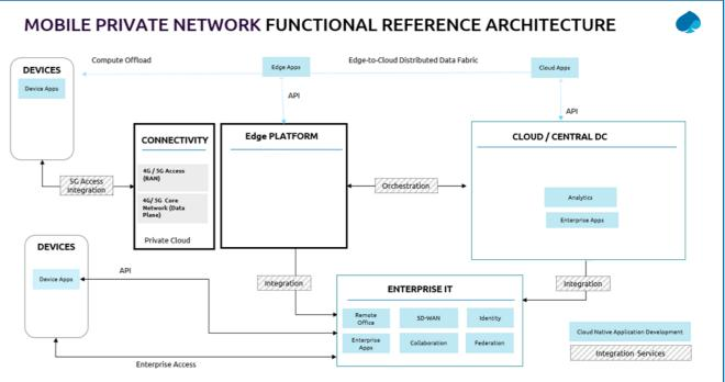
In the second, the architecture can be disaggregated, with 5G RAN and UPF onsite for low latency processing, and the rest hosted in a service provider's cloud.
